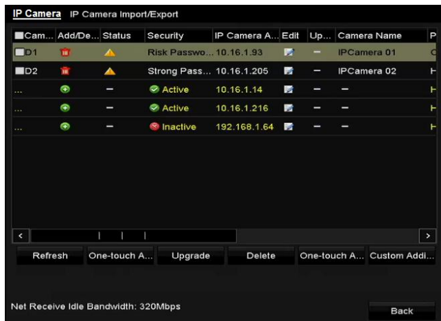
Figure 2. 16 IP Camera Management Interface
